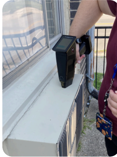
A Lead Risk Assessor uses an XRF analyzer to determine if lead is present in a painted surface.
