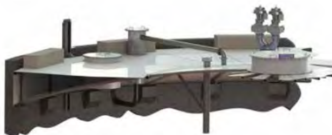
Figure 11-21. Example Radial Beam-Type Floating Digester Cover
