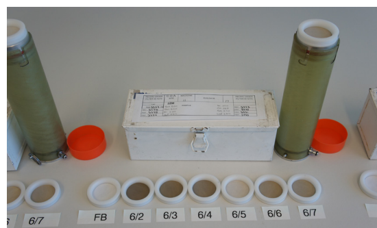
Figure 3. Filters retrieved from air sampling equipment located in the Albuquerque area during the 2011 Arizona Wallow Fire. The filters are either labeled FB (field blank for reference) or by sample date (6/2-6/7). Photo by Erik Bacon
