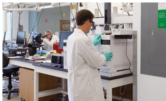
Terry Cain, IA SHL environmental laboratory supervisor, works at a Gas Chromatograph/Mass Spectrometer analytical system to test environmental samples. Photo by Pat Blake
