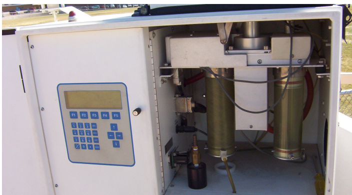
Figure 5. Air particle sampler interior showing the filter cassettes used to load and unload filters from the air flow mechanism. Photo by Albuquerque Department of Environmental Health
