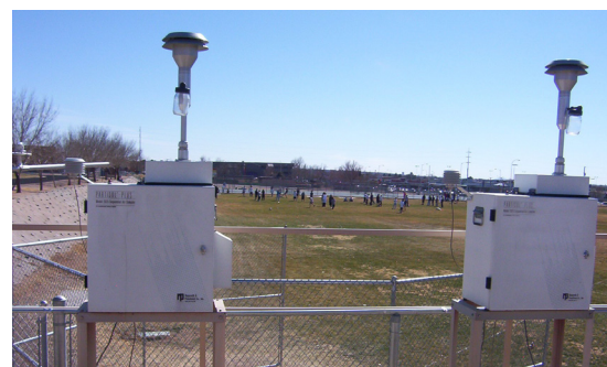
Figure 4. Air particle samplers located in the Albuquerque area. Photo by Albuquerque Department of Environmental Health
